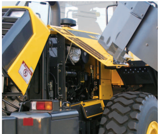
Gull-wing side doors lower stop position
