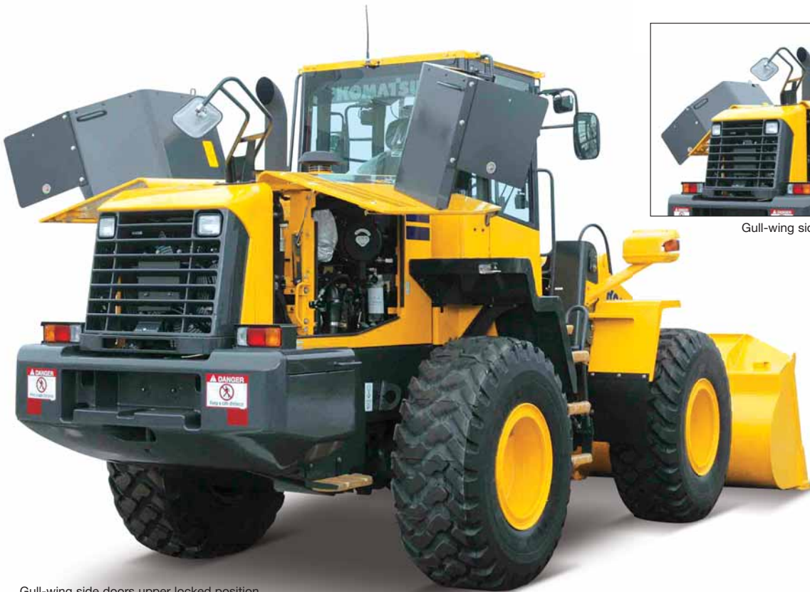
Gull-wing side doors upper locked position
