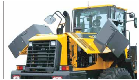
Gull-wing side doors lower locked position
