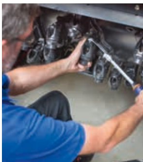
Only 100 Nm bolt tightening torque needed when changing the holder
