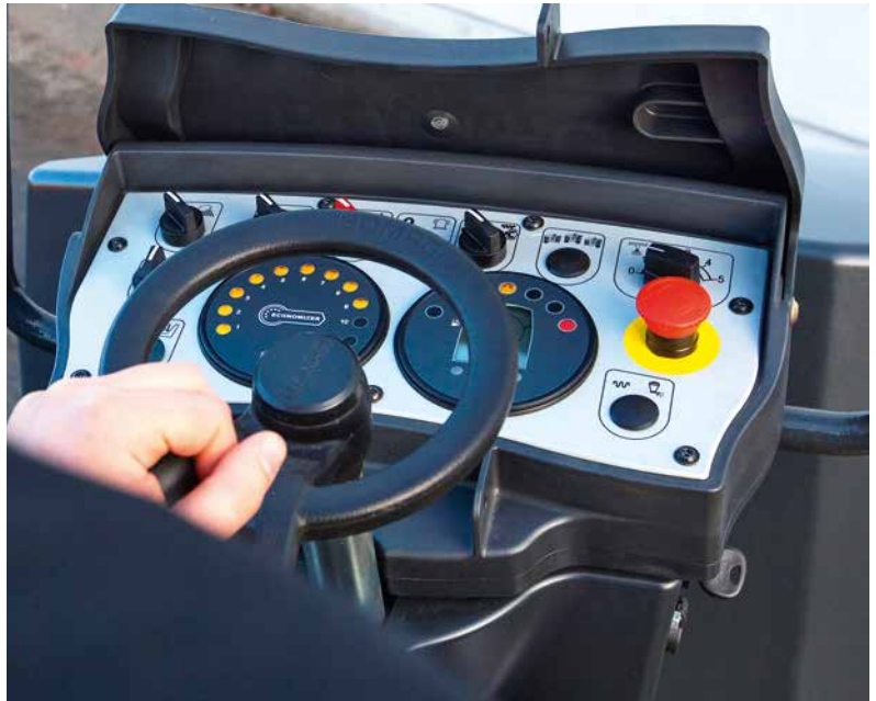
Large switches, a compact steering wheel and clearly arranged control elements make it easy for any operator to work with a light BOMAG tandem roller.
