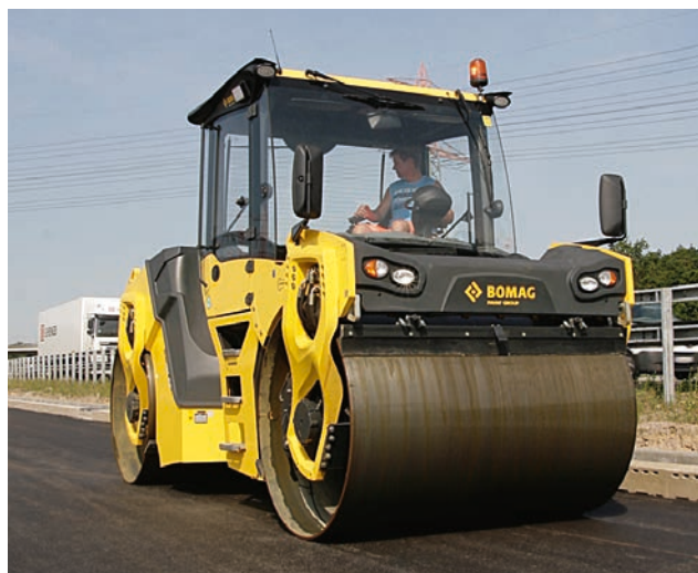
BW 191 with its wide drums is ideal for high volume output and static rolling.
