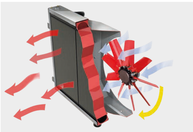
Reversible fans for less cleaning and greater utilisation.
