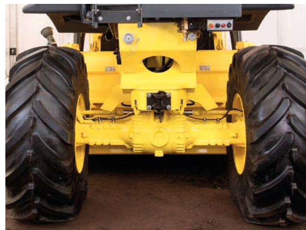
Non-spin oscillating axle \pm 15^\circ (RS 460).
