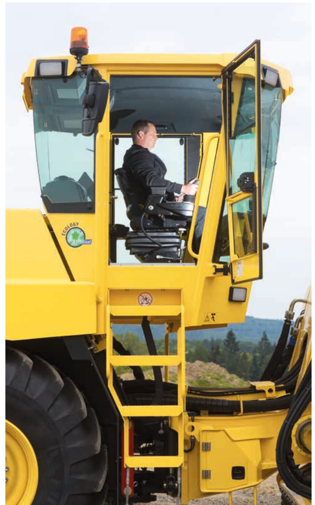
Perfect view even in reverse travel with the 270 degree rotating seat.
