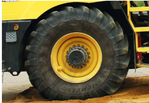
Large wheels for low ground contact pressure.
