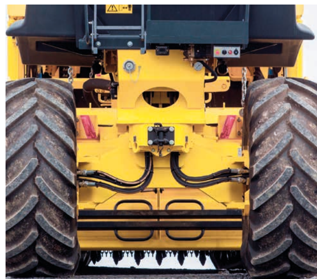
Rear axle with powerful single drives (RS 500).
