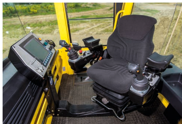
The display is for displaying and setting only the metering systems.
