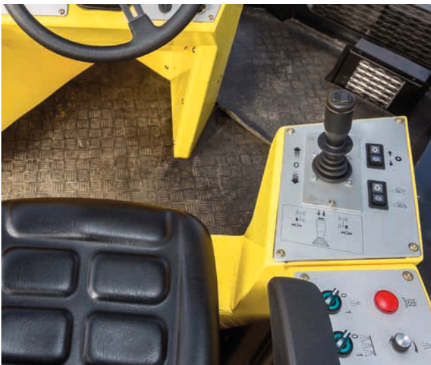
Travel lever and single-wheel brake on the rear axle to provide more precise manoeuvrability.
