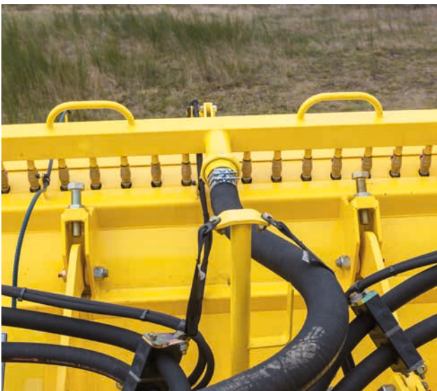
Flexible: 17 injection nozzles switchable on and off on an individual basis.
