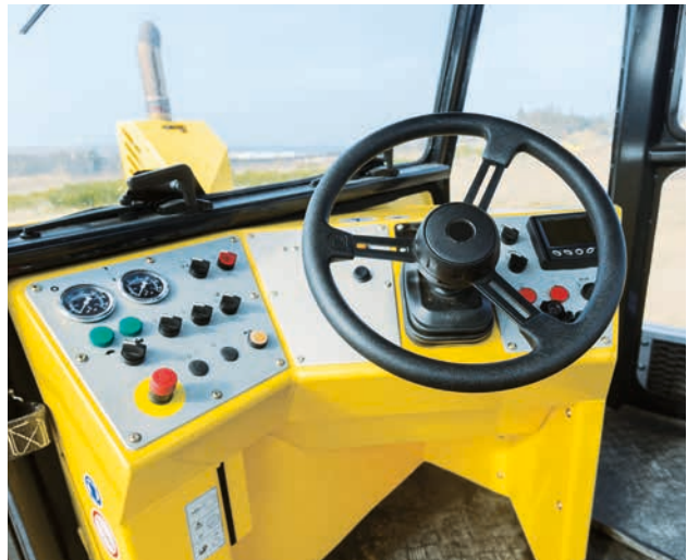
Hydraulically supported steering for more mobility on-site.
