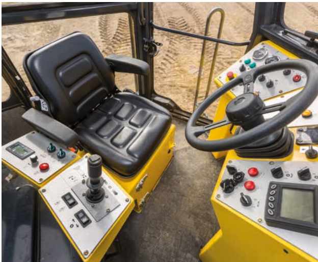
Driver's seat arranged at an angle to provide an ergonomic sitting position and reduces strain.
