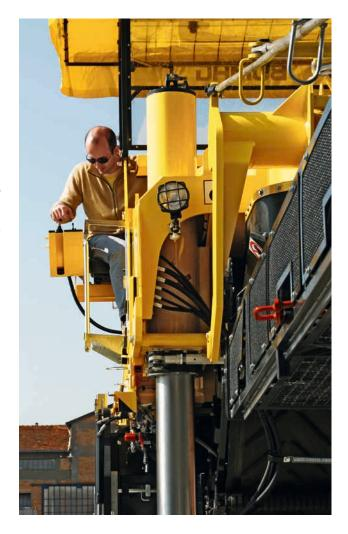
The driver's seat, which can be shifted outwards, a vibration insulating step and a comfortable arm rest, with the most important functions integrated, enable the driver to follow winding country roads with precision and reduced fatigue.
