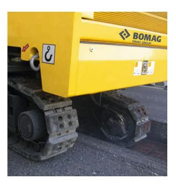
For sewer work wearing, binder and bearing courses can be removed in one pass. The optimal weight distribution ensures excellent traction and directional stability.
