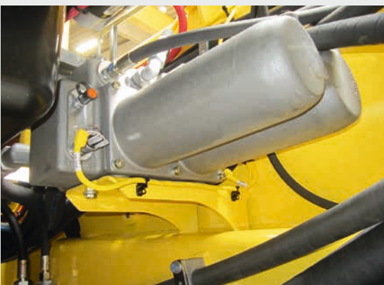
Electronic monitoring of hydraulics return filter system.
