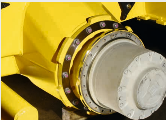
Two independent braking systems (hydrostatics used for service brake, multiple discs for the parking brake).
