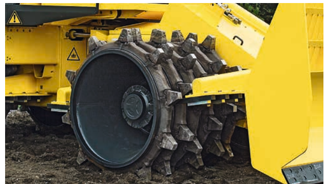
Welded wheel bodies with inner taper on both sides for optimum stability (premium).
