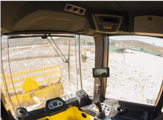
Cab with large windcreens to ensure the best overview of the working environment.
