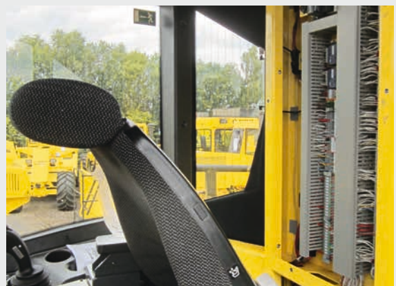
Well protected control centre in the cab.
