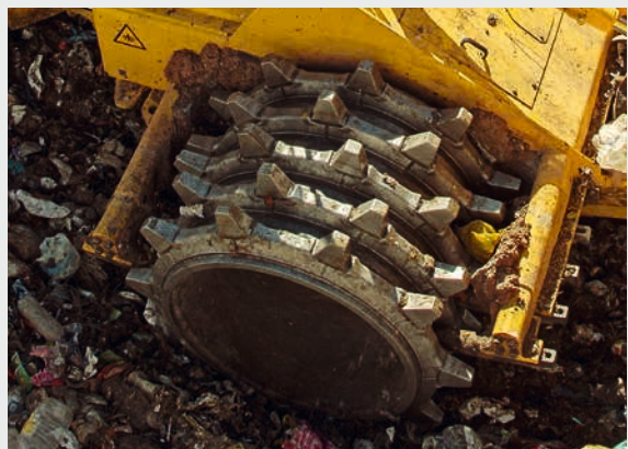
Clean wheels with effective scrapers (optimum compaction).
