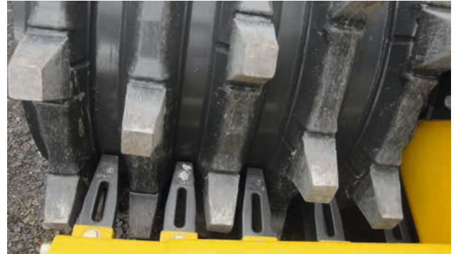
Adjustable scraper for uninterrupted operations.
