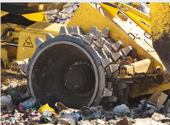
Scrapers guarantee clean wheels and high compaction.
