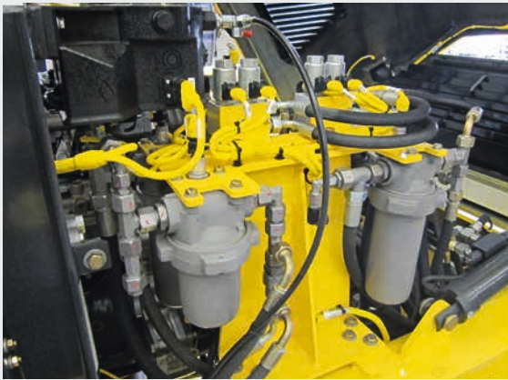
Discharge side of the hydraulic filter system.
