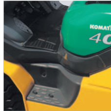
Improved design of engine hood and step
