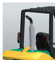
Upward exhaust muffler
