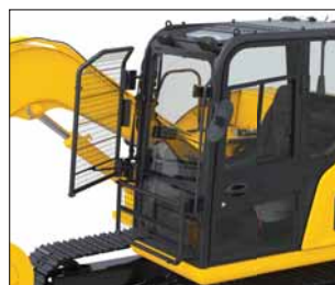
Cab front full height guard, OPG level 1 (ISO 10262)
