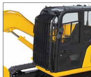
Cab front full height guard, OPG level 2 (ISO 10262)
