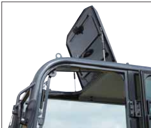
Large roof window
