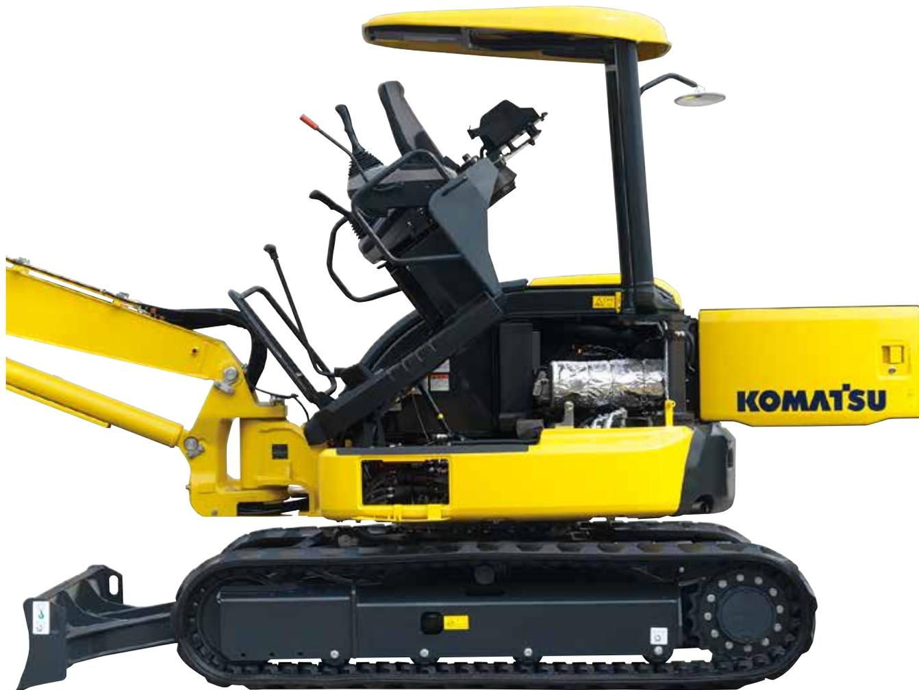
Thermal and Fan Guards are Placed Around High-temperature Parts of Engine and Fan Drive
