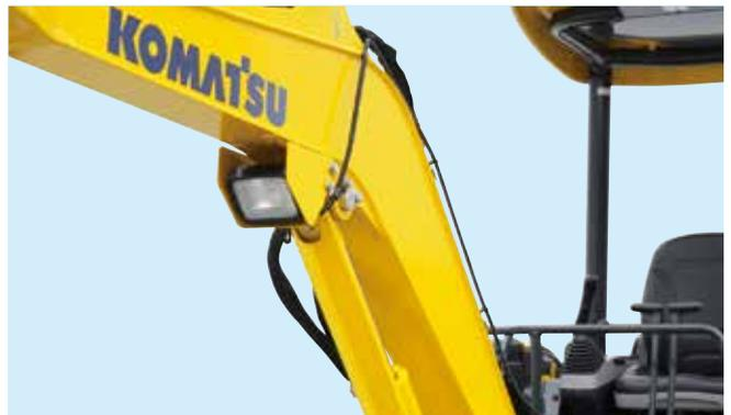
This travel lamp provides an increased visibility both in a night operation and in the travel position.
