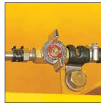
Fuel drain valve
