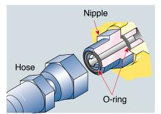
Flat face-to-face O-ring seals are used to securely seal all hydraulic hose connections and to prevent oil leakage.
